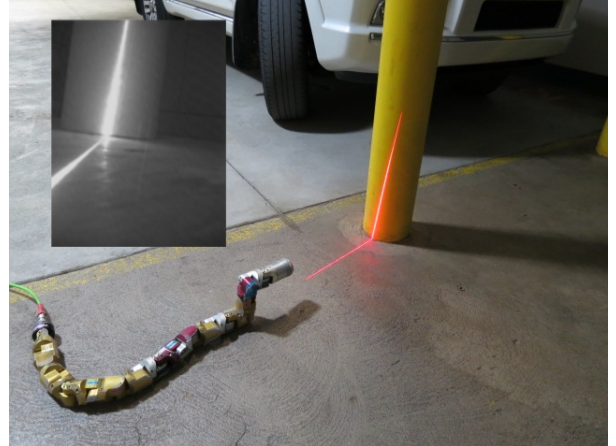
Fig. 1: Modular Snake scanning the environment. The snake is partially curled to have a stable position. The snake head is lifted up to have a better viewing point and to allow the head to freely scan. The red line is the light from the laser. The inset shows the camera image (rotated for clarity).
