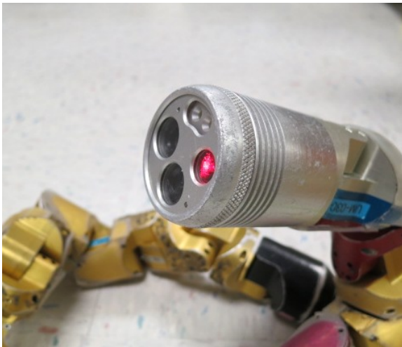
Fig. 2: Sensor head on the CMU modular snake robot. A red laser is on the right and a B/W camera is on the left. They form the structured light sensor. On the bottom is a color camera and on the top are two LEDs for illumination.
